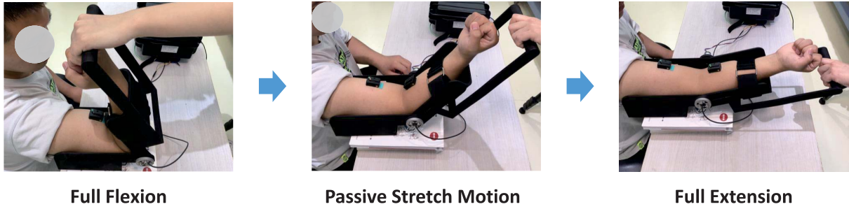
Fig. 3. Overview of the experimental setup. For each subject, the initial position of the elbow joint was defined as the maximum flexion allowed by the approximation of the upper-arm and the forearm, and the final position was defined as the maximum extension of the joint. The spasticity phenomenon in the elbow flexors and extensors was evaluated by stretching the handle to make the joint passively move from the initial position towards the final position at an arbitrary velocity.
