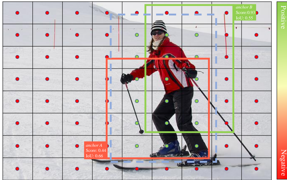
Figure 1: Illustration of the defects of the conventional label assignment in current one-stage detectors. They suffer from two major limits: (1) Misalignment between assignment strategy and NMS procedure. (2) Rigid sample assignment during training process.
