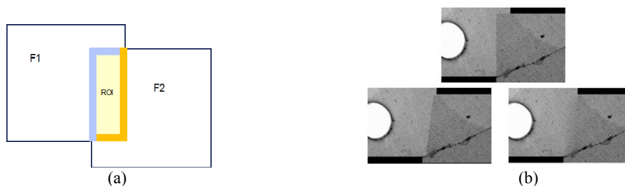
Fig.3. (a) The mosaicked model image of using Poisson image editing. (b) Original Mosaicked EM image (up) and the result contrast of multiresolution image blending (left) and Poisson image editing (right).
