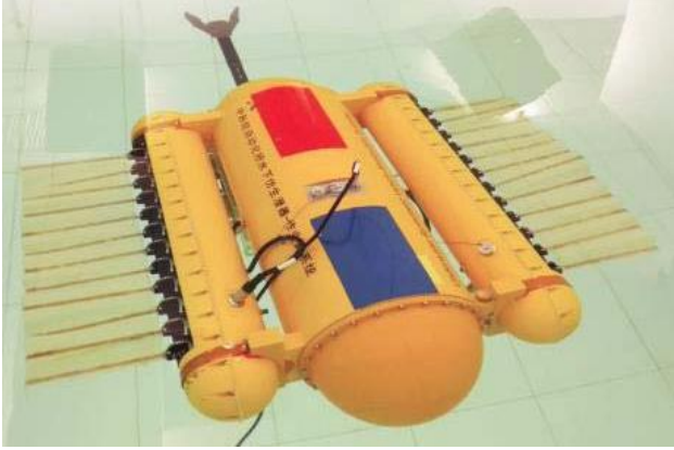
Fig. 1 Biomimetic underwater vehicle (RobCutt-II)
