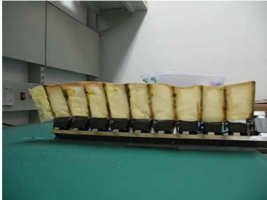
Fig.5. Ribbon-fin mechanism used in the experiments
