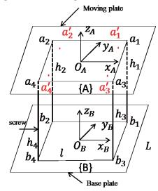
Fig. 4 Simplified architecture for parallel mechanism
