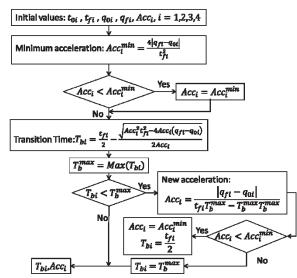
Fig. 7 Flow chart of linear interpolation with parabola transition
