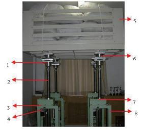
Fig. 2 Parallel mechanism for each moving plate (1 – spherical component, 2 – vertical screw, 3 – planetary reducer, 4 – step motor, 5 – top moving plate, 6 – two-dimensional translational component, 7 – screw nut with gear teeth box, 8 – base)
