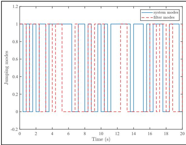
Figure 1. The jumping modes of Markovian jump system and its filter.
