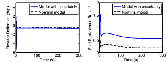
Fig. 3. Control inputs:  $\delta_e$  and  $\beta$ .
