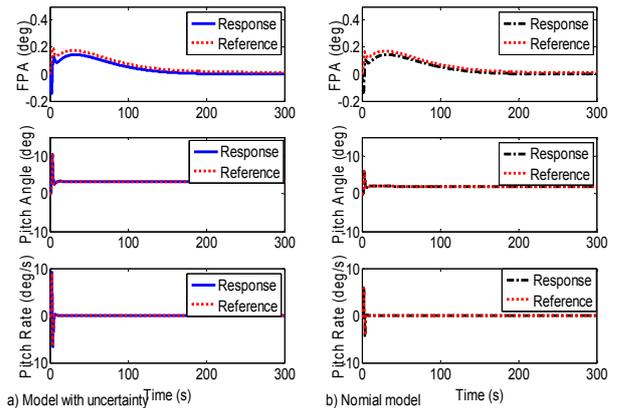
Fig. 2. Tracking performance of FPA, pitch angle and pitch rate: a) Model with uncertainty, b) Nominal model.
