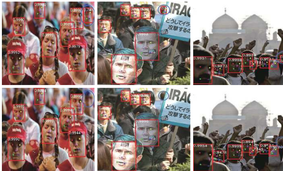
Fig. 9 Comparison of visual results with and without the attention module. The top row shows the detection results without the attention module, and the blue circles represent the parts of error detection. The bottom row shows the detection results with the attention module added, and the blue circles represent the parts of correct detection.
