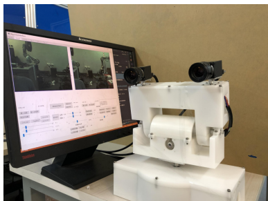
Fig. 3. Active stereovision platform.
