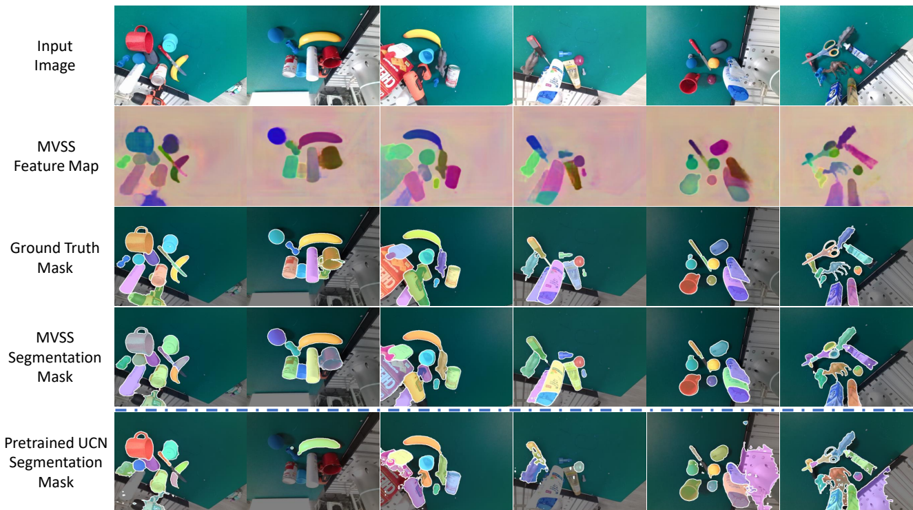
Fig. 5. Examples of the feature maps and segmentation masks obtained by MVSS and UCN pretrained on TOD [20]. It is observed that the pre-trained UCN yields mis-segmented samples in real-world scenes, even only a few objects can be correctly segmented in some scenes. Incorporating our proposed MVSS framework, the network is able to utilize multi-view observations for self-supervised feature embedding learning, achieving improved accuracy and consistency without the need for annotations.
