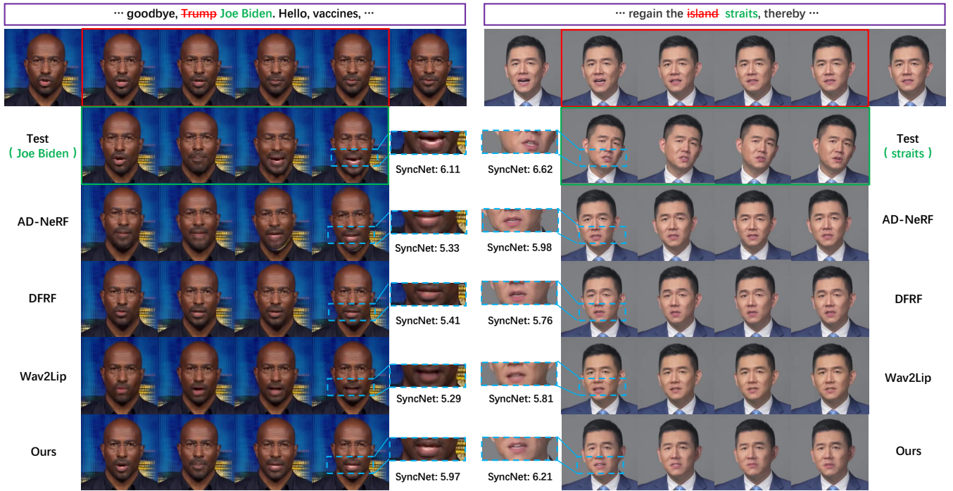
Figure 3: The results of substituting the word of the talking-head videos. We further evaluate the SyncNet [9] scores of the edited video clips.
