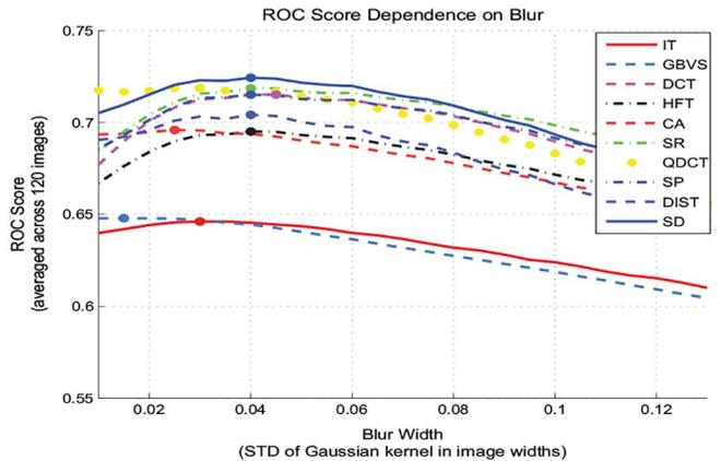
Fig. 4. ROC Area Under the Curve (AUC) Score. This metric follows the procedure proposed on the benchmark [11]. The curves show that our model SD outperforms the other models on predicting human fixations.
