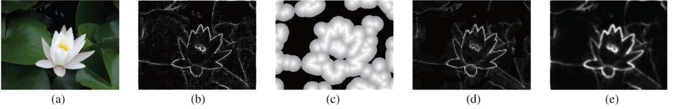
Fig. 2. Illustration of the main phases of our model. (a) Input an image. (b) Calculate the sparse saliency at first. (c) Get the candidate regions. (d) Calculate the distinctive saliency in the candidate regions. (3) Integrate sparse and distinctness saliency for the final saliency map.
