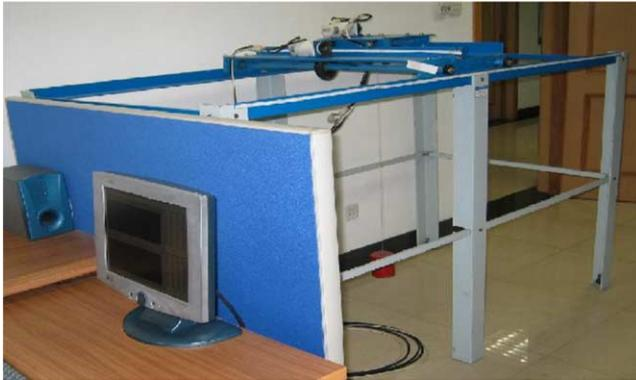
Fig. 4. Two-dimension prototype overhead crane.
