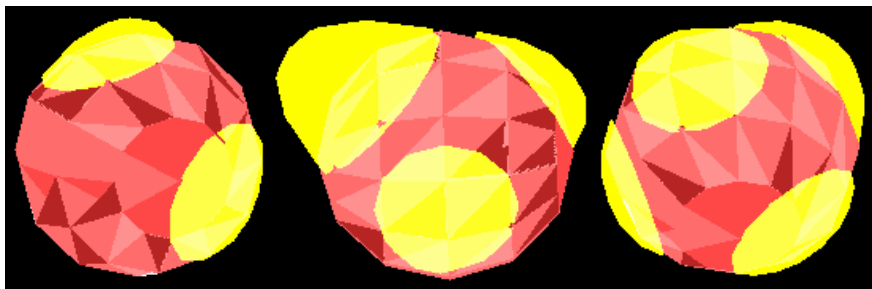
Figure 7 Three views of the original bioluminescent sources (the solid sphere) and the local surface modified by the Bezier cubic spline curves (the local convex surfaces)
