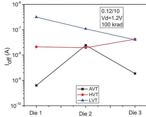
Fig. 3. Post-irradiation  $I_{off}$  of different process variants from three different die.
