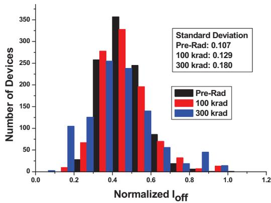
Fig. 5. Histogram plot of leakage current for a NMOS transistor with  $W=0.12 \mu\text{m}$ ,  $L=0.08 \mu\text{m}$ .
