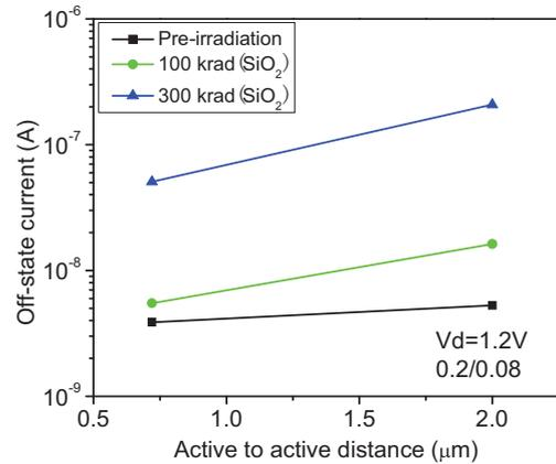
Fig. 7. Pre- and post-irradiation off-state current evolution with active to active distance.
