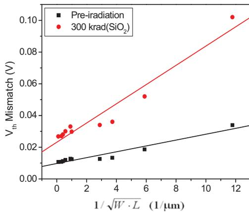
Fig. 6. Pelgrom plot of linear  $V_t$  mismatch for NMOS transistors.
