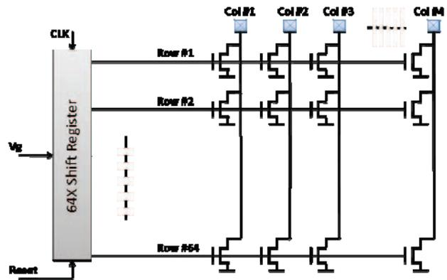
Fig. 1. Transistor array schematic circuit diagram.
