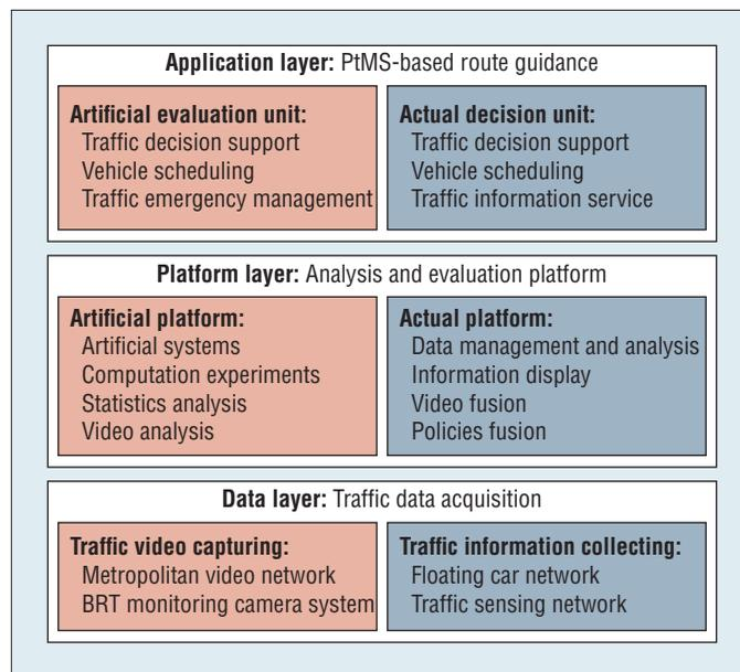
**Figure 3. The parallel traffic management system (PtMS) system architecture and main functionalities for the 2010 Asian Games. The system consists of three layers: data acquisition, operational platforms, and traffic applications.**
