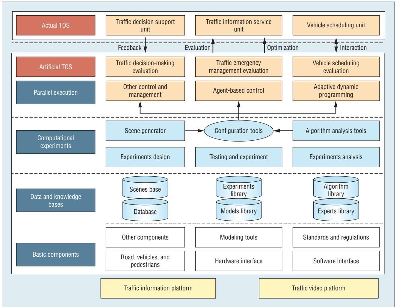
**Figure 4. System architecture of parallel traffic management system (PtMS) based route guidance. The actual transportation operation system (TOS) supplies traffic information distribution and guidance generation, and the artificial TOS helps with traffic scenario generation, decision testing, and effectiveness evaluation.**
