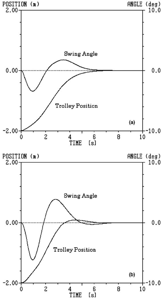
Fig. 8. Control simulation example (4). (a) Proposed fuzzy controller, (b) linear state feedback controller.
