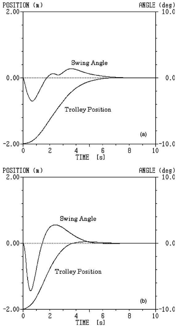
Fig. 7. Control simulation example (3). (a) Proposed fuzzy controller, (b) linear state feedback controller.
