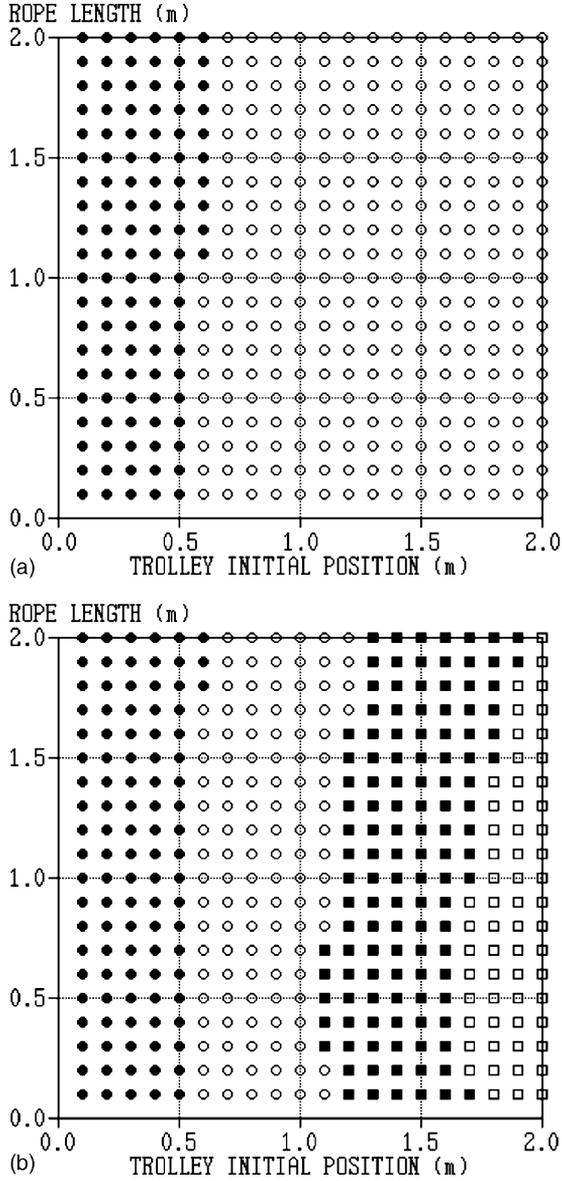
Fig. 10. Comparison of maximum swing angles. (a) Proposed fuzzy controller, (b) linear state feedback controller.
