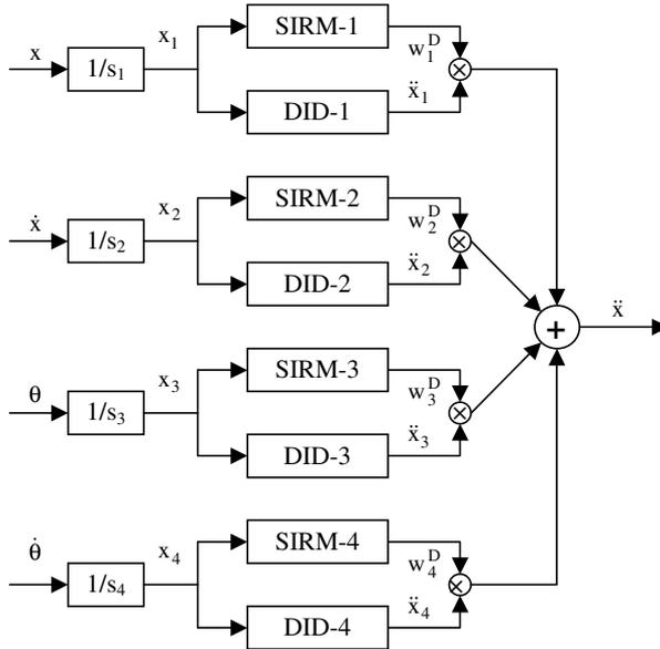
Fig. 4. Block diagram of the fuzzy controller.
