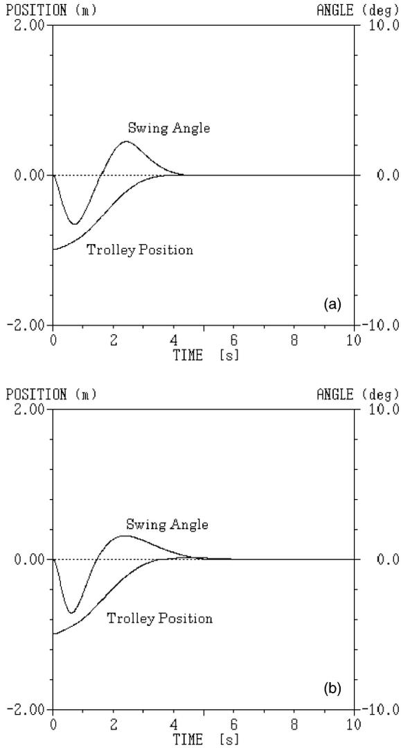
Fig. 5. Control simulation example (1). (a) Proposed fuzzy controller, (b) linear state feedback controller.
