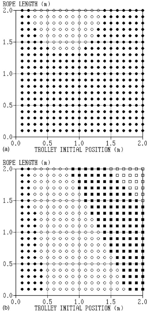
Fig. 11. Comparison of overshoot amounts. (a) Proposed fuzzy controller, (b) linear state feedback controller.
