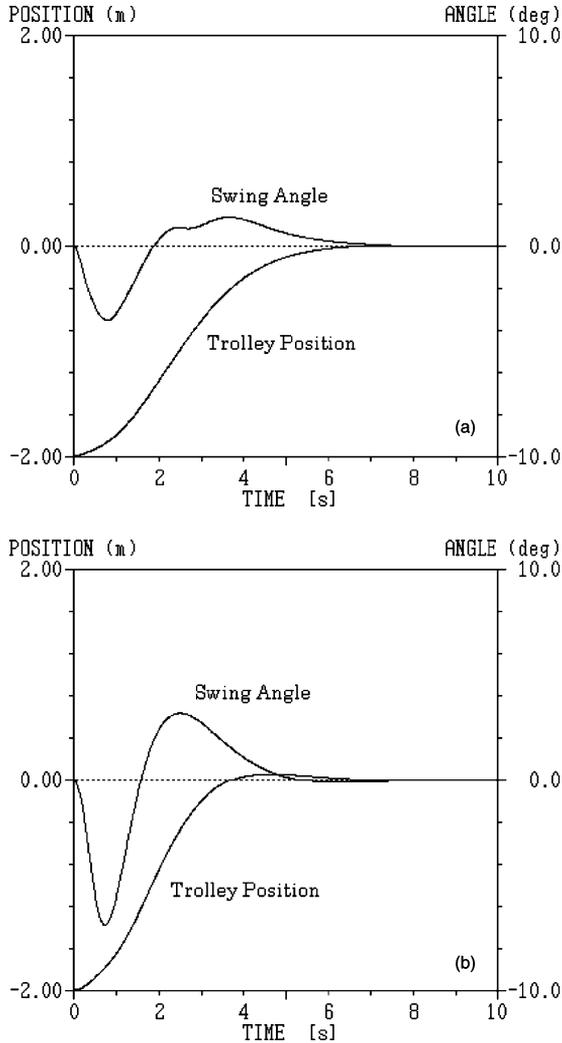
Fig. 6. Control simulation example (2). (a) Proposed fuzzy controller, (b) linear state feedback controller.
