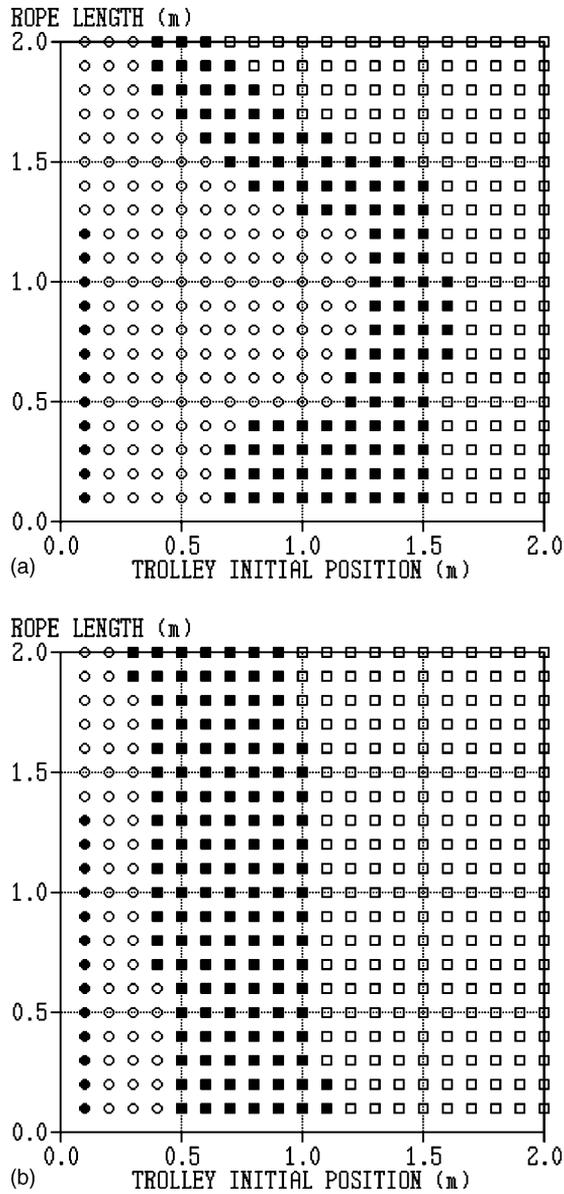
Fig. 9. Comparison of transportation time. (a) Proposed fuzzy controller, (b) linear state feedback controller.
