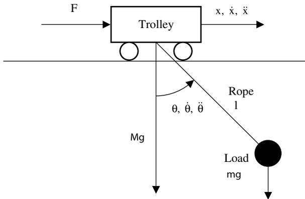
Fig. 1. Overhead traveling crane model.
