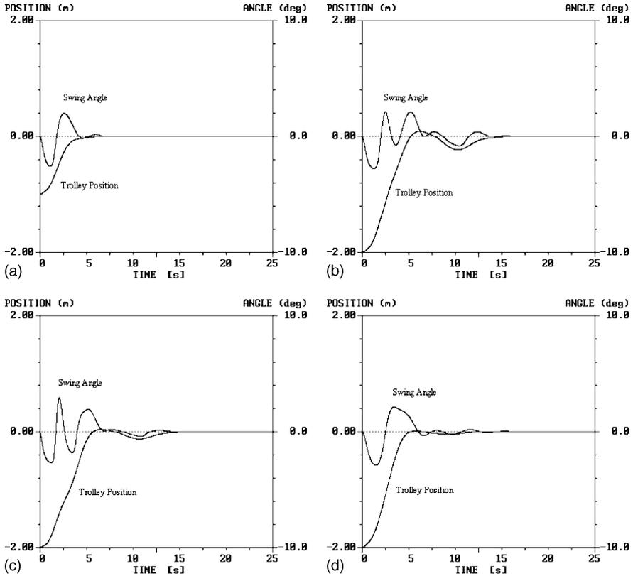
Fig. 12. Simulation results by traditional fuzzy controller. (a) Rope length 1.0 m and trolley initial position  $-1.0$  m, (b) rope length 1.0 m and trolley initial position  $-2.0$  m, (c) rope length 0.5 m and trolley initial position  $-2.0$  m, (d) rope length 2.0 m and trolley initial position  $-2.0$  m.
